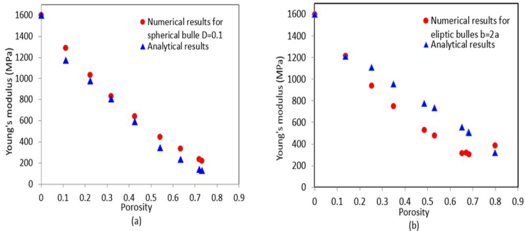
Fig.7.Comparison of numerical results with analytical resultsfor (a) the spherical model, (b)the elliptic model
