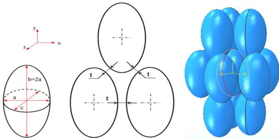
Fig 2.Dimension (left)and arrangement (right)of elliptic cells
