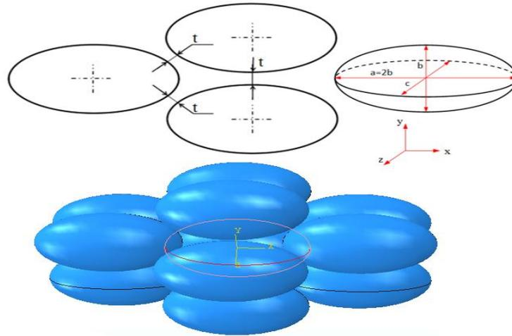
Fig 3.Dimension (left)and arrangement (right)of elliptic cells
