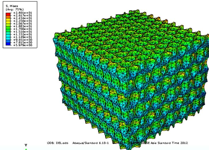
Fig.5. Von Mises stresses for the RVE
