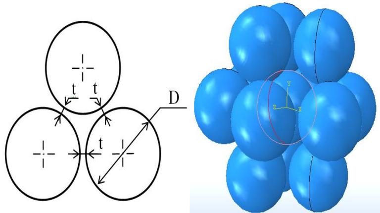
Fig 1.Dimension (left)and arrangement (right)of spherical cells
