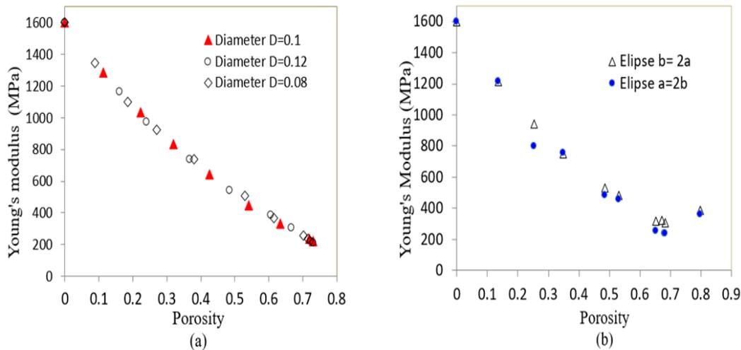
Fig.6. The relations between the Young's Modulus and the Porosityfor (a) the spherical model, (b)the elliptic model
